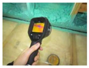
The main advantage of the midconstruction (pre-drywall) test is that air leakage / thermal issues can be easily addressed prior to completion (As-Built).
