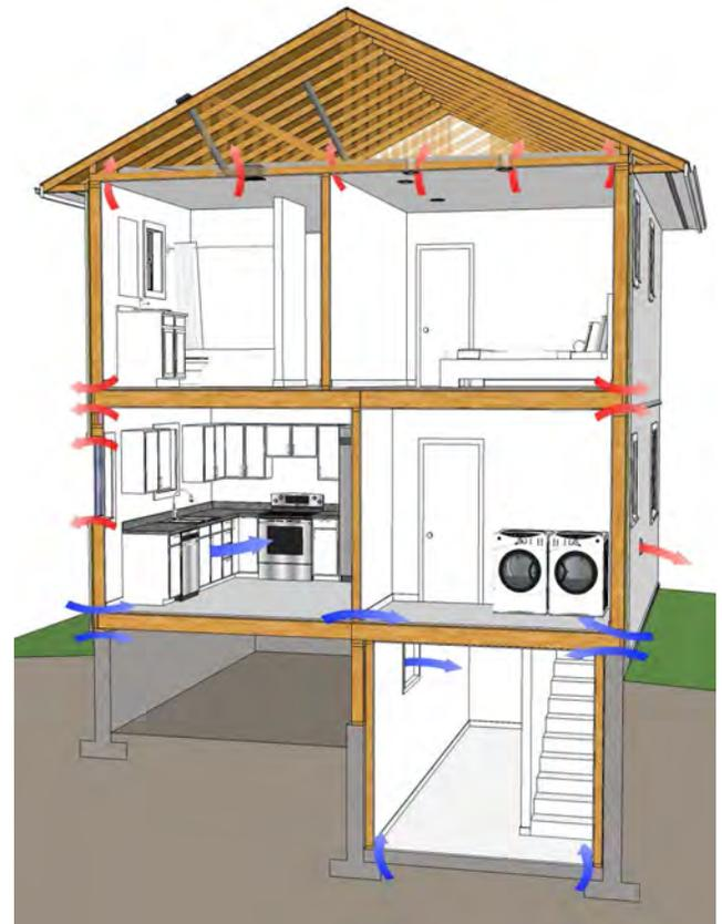
*Schematic of a typical two-storey wood-frame house over part basement and crawlspace with a ventilated attic roof. Arrows show typical air leakage locations to review and address during weatherization work.*
