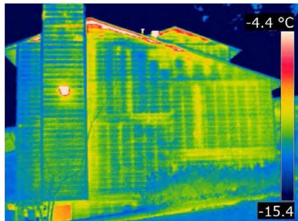
*Infrared images such as this, showing a wood-frame home in B.C., can identify insulation discontinuities and air leakage locations, which can assist contractors with weatherization retrofits.*
