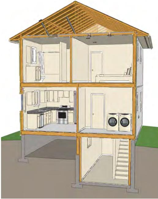
*All the parts of the house including its contents and occupants interact together to form an integrated system - this is imperative to understand when performing air sealing and insulation work. This guide covers air sealing and insulation weatherization work for all parts of the house from the basement to the attic.*
